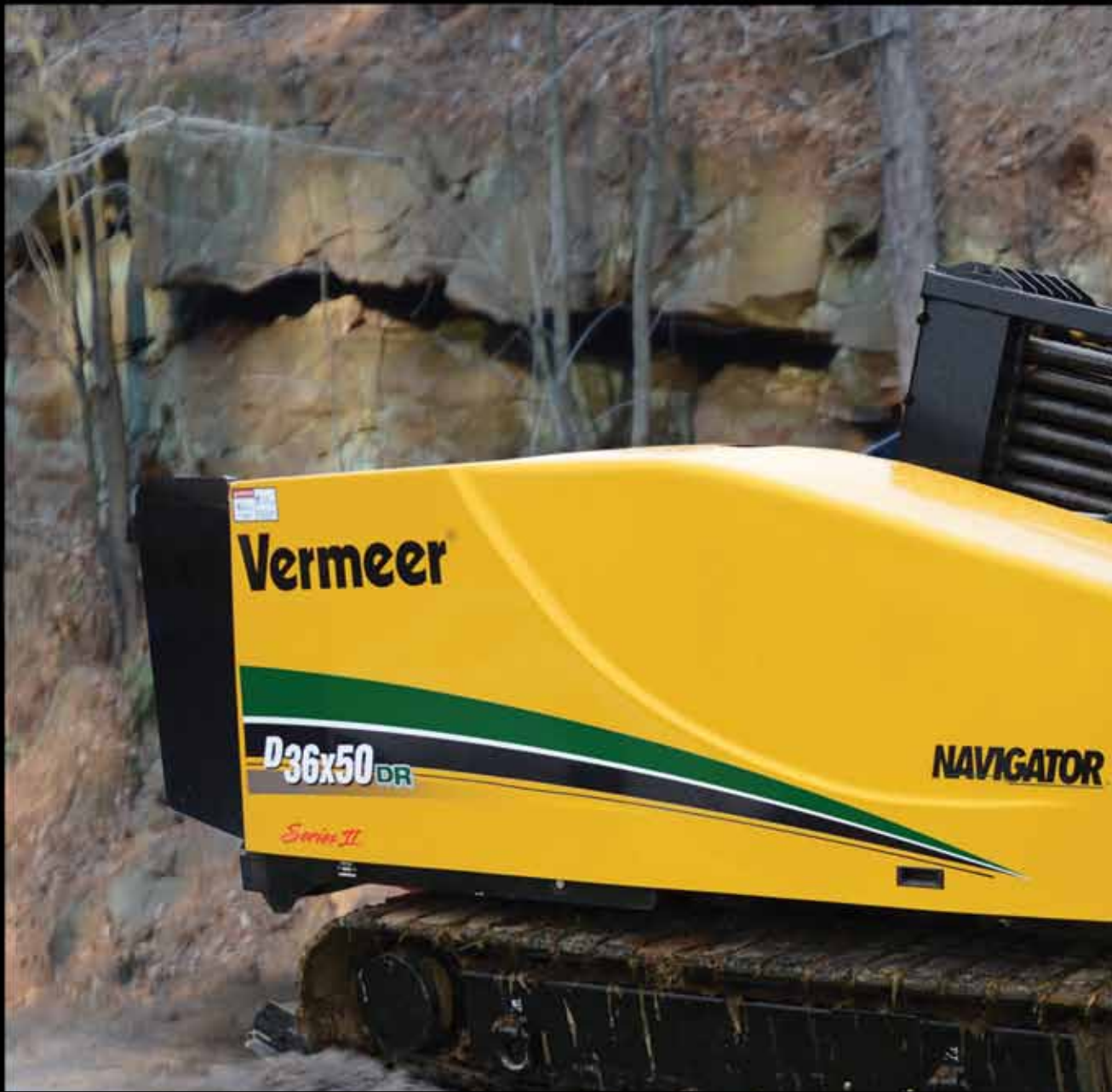
4: Rod carrying capacity. The D36x50DR Series II carries up to 500' (152.4 m) of drill rod, reducing the need to load additional rod when performing extended bores.
