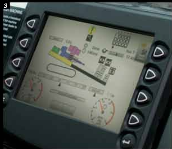
3: Makeup or breakout? Controls provide options including automated sequence, partially automated sequence or manual sequence of the rod makeup/breakout process depending upon operator preference and level of expertise.
